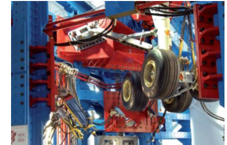
Landing Gear Dynamics Test
